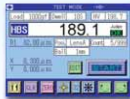
Light-load brinell mode
