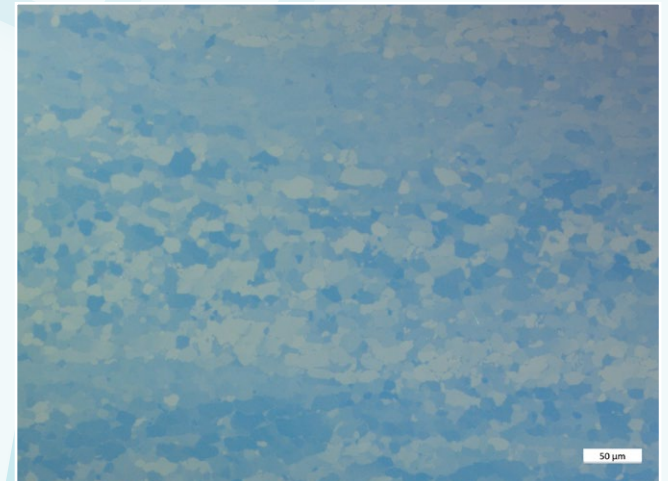
Pure Titanium, Grade 2, POL + Lambda Compensator, 200x
