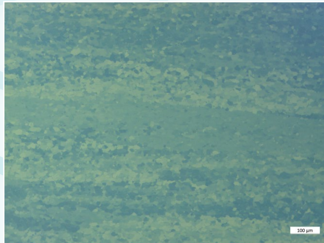
Pure Titanium, Grade 2, POL + Lambda Compensator, 100x
