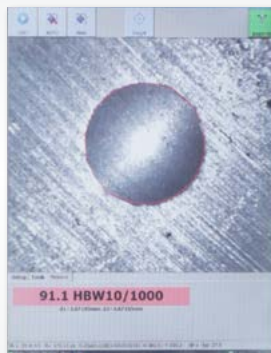
Clear view of the indent and the tested area
