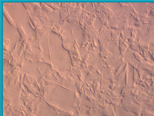
Copper, DIC, 200x after polishing with Fumed Silica, Alkaline, with additives, on Chermal.
