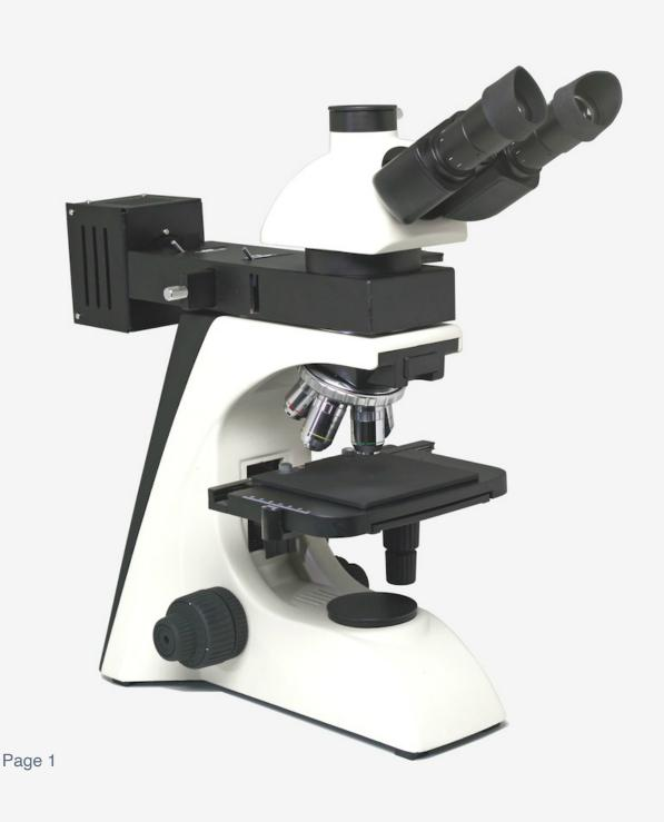
The Microtec RM-1-MET with its 12V 50w incident illuminator has a field iris diaphragm and an aperture diaphragm, enabling the illumination to be optimally adjusted at all magnifications.
