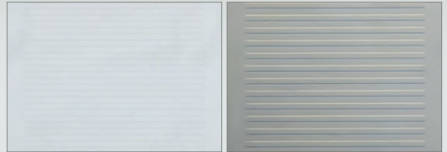
Conventional diascope illumination OCC illumination
