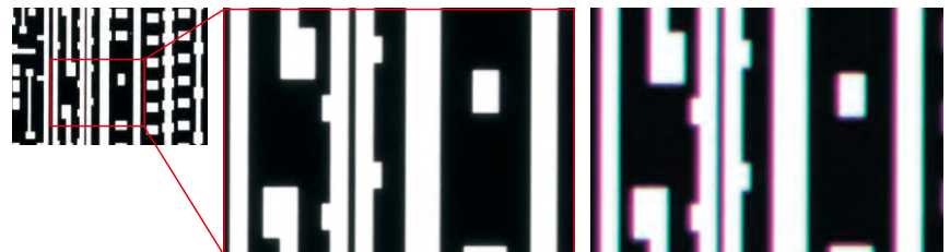
Apochromat optics (captured with SMZ1270+Plan Apo 1x/WF)
