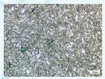
Low Alloy Steel 42CrMo4+QT, 330 HV etched with Nital 3%, BF, 1000x
