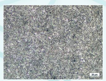
Low Alloy Steel 42CrMo4+QT, 330 HV etched with Nital 3%, BF, 500x
