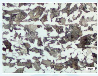
0.45% C Steel, normalised, 200 HV, longitudinal section etched with Nital 3%, BF, 500x
