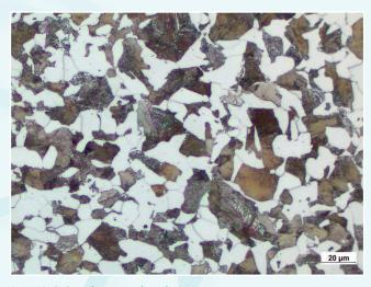
0.45% C Steel, normalised, 200 HV, cross section etched with Nital 3%, BF, 500x
