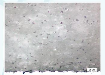
$Al_2O_3$  coating on a steel substrate, BF, 500x
