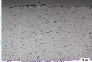
Al<sub>2</sub>O<sub>3</sub> coating on a steel substrate, BF, 200x
