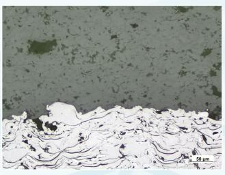
Thermal barrier coatings with ceramic top and metallic bond, BF, 200x
