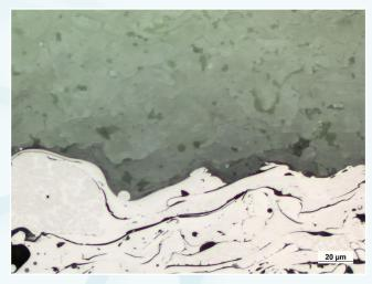
Thermal barrier coatings with ceramic top and metallic bond, BF, 500x
