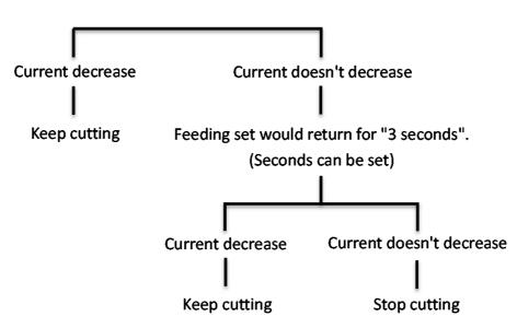
When current  $\geq$  AL1: Stop feeding for 3 seconds
