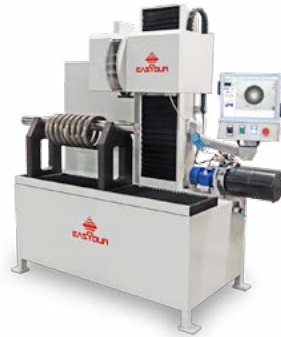
INTEGRAL SPRINGS on cylinders and bottles. Built-in programmable milling.
