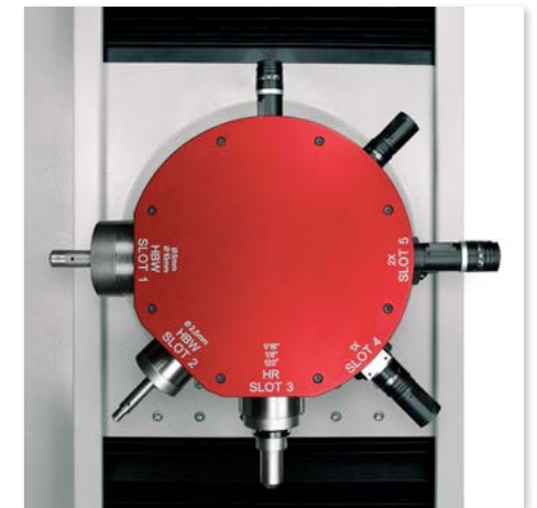
Motorized turret 8 positions
